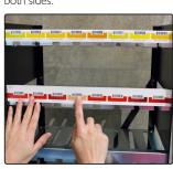
/. Repeat with remaining rackstrips working your way to the bottom shelf. This completes assembly for one rack.
